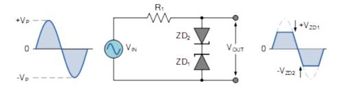
The output waveform from full wave zener diode clipping circuits resembles that of the previous voltage biased diode clipping circuit. The output waveform will be clipped at the zener voltage plus the 0.7V forward volt drop of the other diode. So for example, the positive half cycle will be clipped at the sum of zener diode,  $ZD_1$  plus 0.7V from  $ZD_2$  and vice versa for the negative half cycle.
