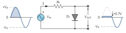
In this diode clipping circuit, the diode is forward biased (cathode more positive than anode) during the positive half cycle of the sinusoidal input waveform. For the diode to become forward biased, it must have the input voltage magnitude greater than +0.7 volts (0.3 volts for a germanium diode).
