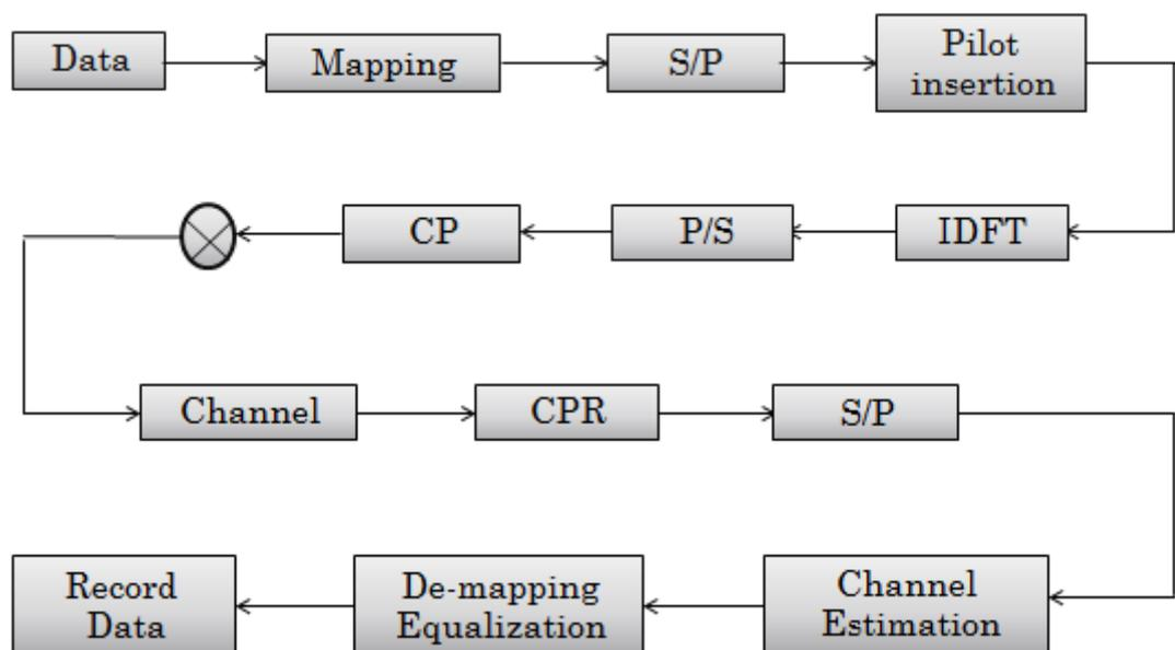
Fig 2.1: Block diagram of OFDM
