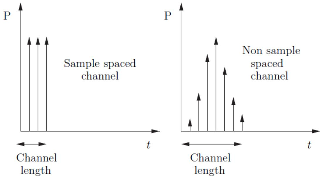
Fig 3.2: Resampling a non-sample-spaced channel extends the channel length.
