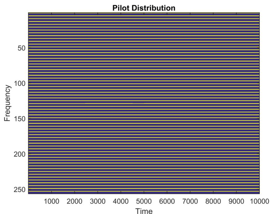
Fig 4.1: Comb-type pilot distribution configuration for 10,000 OFDM symbols.
