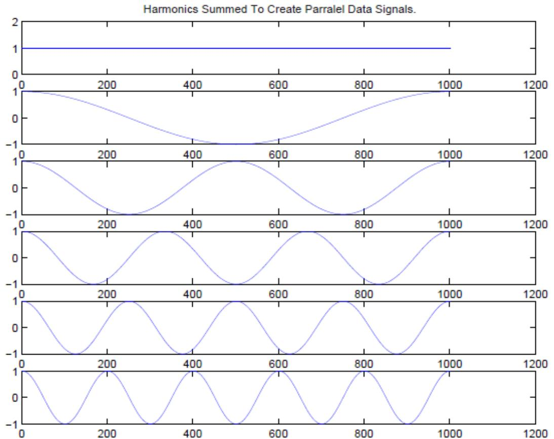
Fig 2.6: Fourier series frequency harmonic
