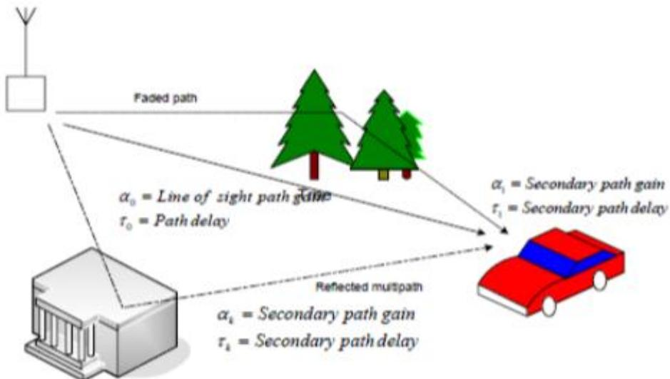
Fig 2.4: Showing the multipath channel
