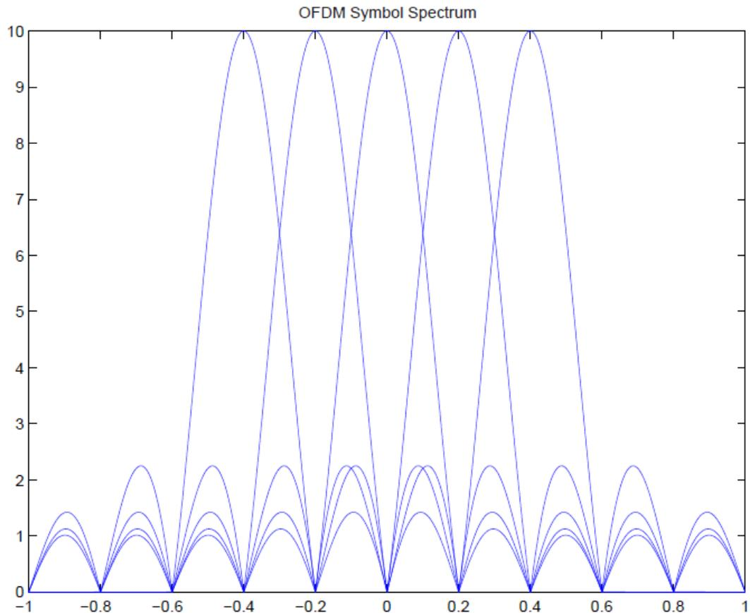
Fig 2.7 : OFDM time domain spectrum
