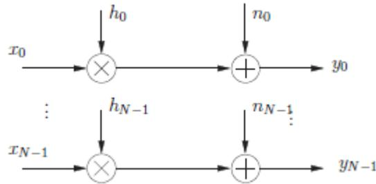
Fig 3.1: Parallel Gaussian channels
