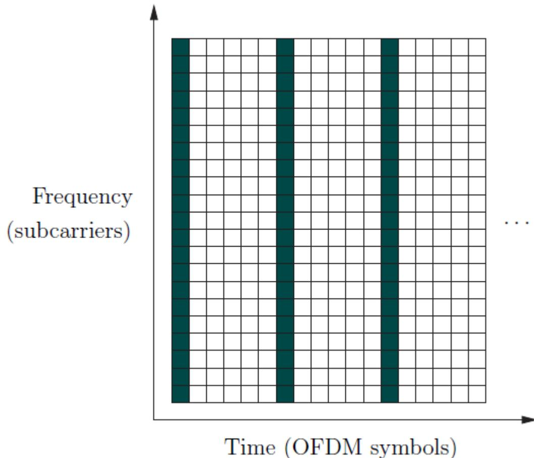
Fig 3.3: An example of block based pilot information
