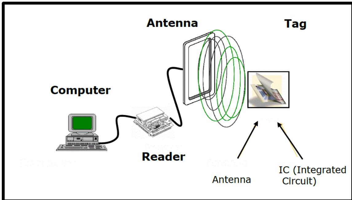
Figure (1.1): RFID construction element
