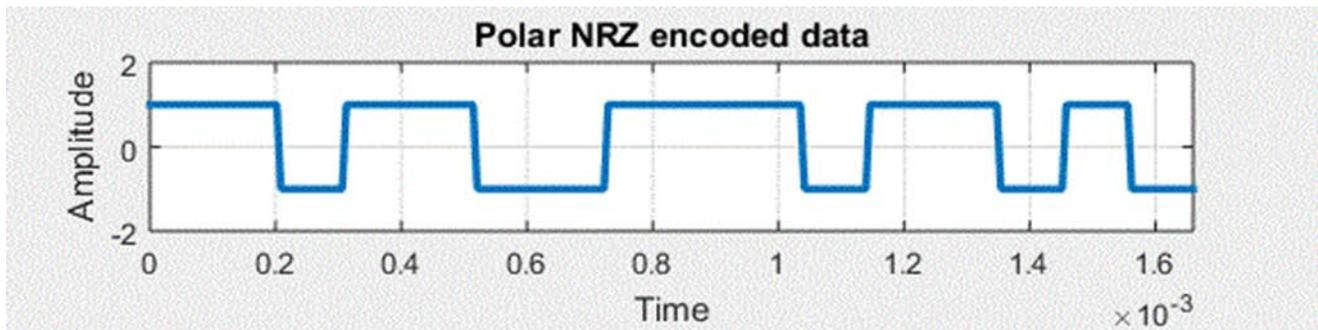
Figure (4.2): polar NRZ line coding for the data in figure 4.1
