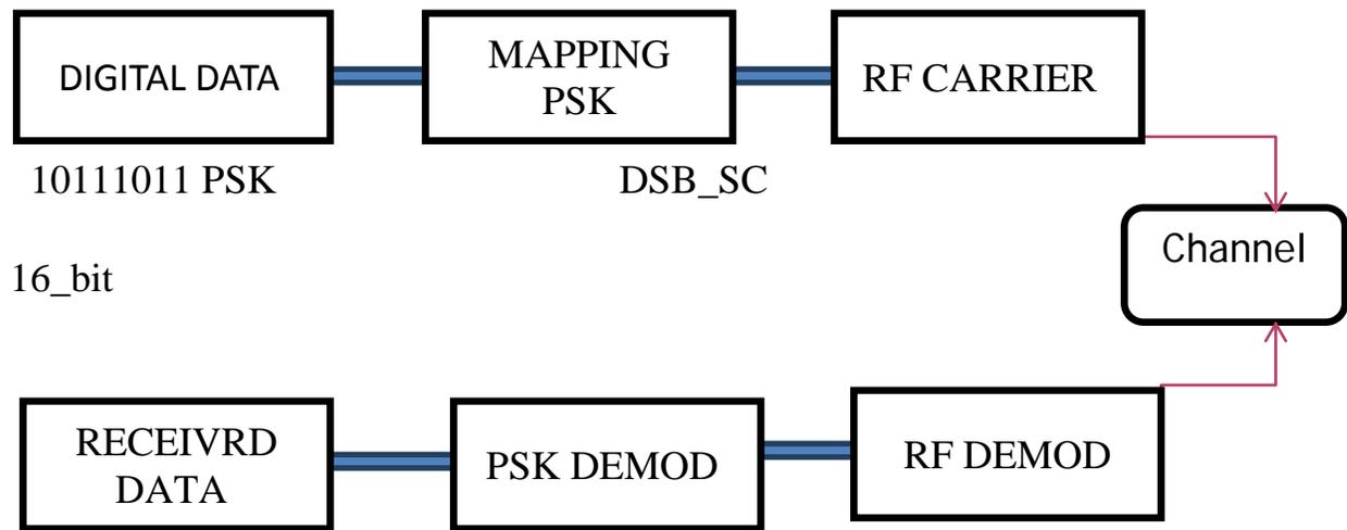
Figure (3.1):A simple block diagram for our RFID system
