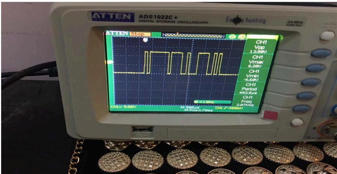
Figure (4.7):DSP\_SC modulated signal
