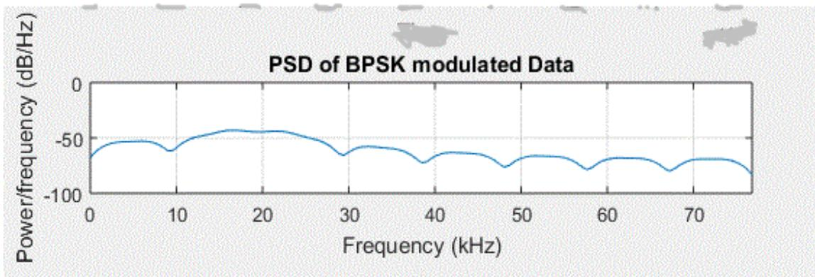
Figure (4.4): power spectral density of the BPSK signal.
