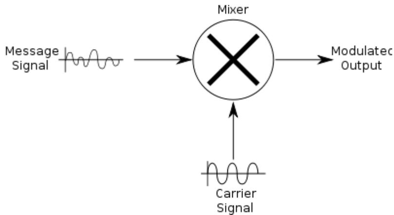
Figure (3.2): DSB\_SC generation using a mixer
