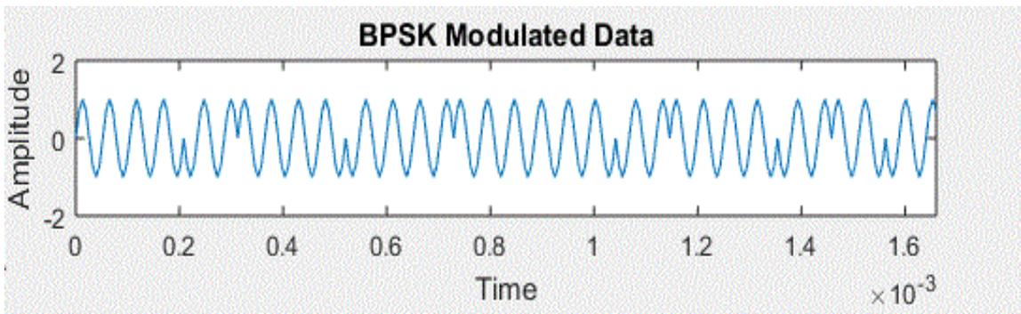
Figure (4.3): BPSK base band modulation.
