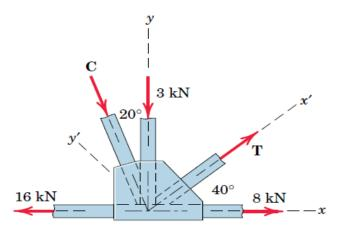
The given sketch constitutes the free-body diagram of the isolated section of the joint in question and shows the five forces which are in equilibrium.
