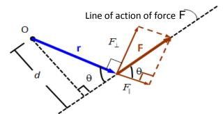
Note: moving a force along its line of action does not change its moment
