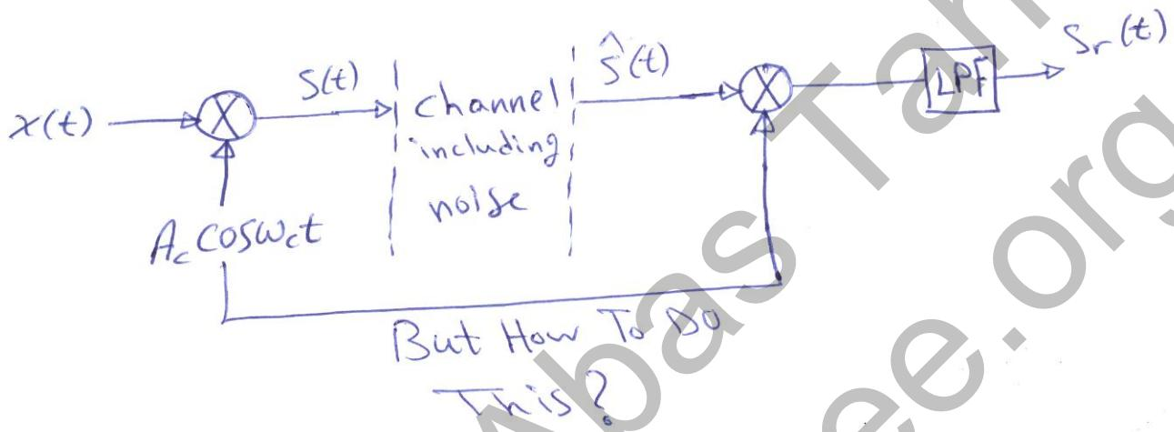
\* The synchronous detector requires two conditions :-
