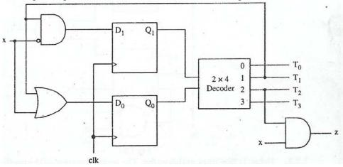
**3.Using one flip flop per state** This method uses one flip-flop per state in the control sequential circuit .Each flip-flop is set at any particular time, while all others are clear .The advantage of this method is simplicity with which it cant designed .The control unit logic can be derived directly from the state diagram without the need of state or excitation tables .The main disadvantage of this method is that it uses a maximums number of flip-flops.
