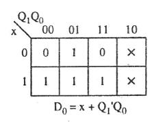
The input functions to the D flip-flops can also be expressed as follows:
